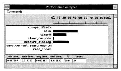
The performance analyzer window shows the name of each function or memory range of each block along with a bar graph showing the percentage of time spent in that function or block. You may select a function to view statistics in the bottom portion of the performance analyzer window. The following statistics are maintained for each function or program block:
