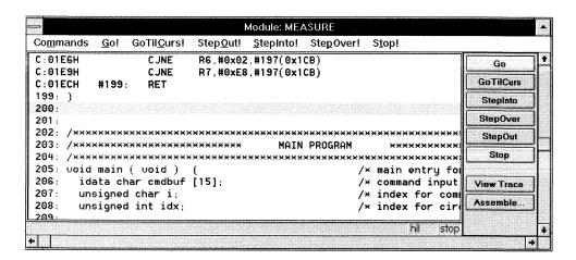
When viewing your application in high level mode, the meaning of a step changes to mean one high-level statement instead of one assembly instruction. Click on the StepInto button and watch as the current program counter line moves down the screen.
