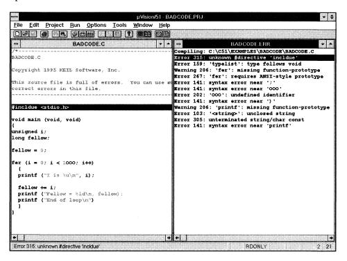
When the error window displays, it may cover a portion of the source window. Use the tile vertical or tile horizontal button to display the windows side-by-side.
