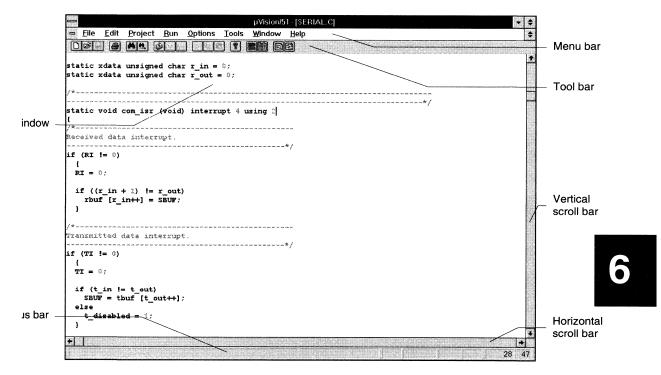
You can quickly access many of the features of  $\mu V$ ision using the buttons on the tool bar.
