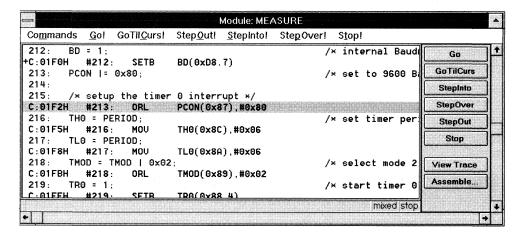
The debug window shows intermixed source and assembly lines.
