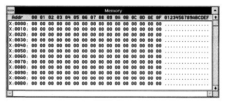
To display the on-chip data memory, enter the following in the command window.
