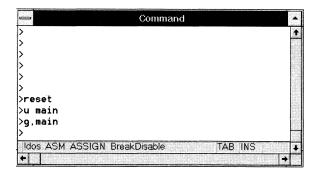
You can interactively display and change variables, registers, and memory locations from the command window. You can also enter assembly code to patch or test parts of your program.
