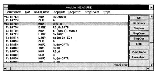
To skip the initialization code and go directly to the main function, select the command window and enter "G,main". dScope executes the startup code and halts on the first statement in the main function.
