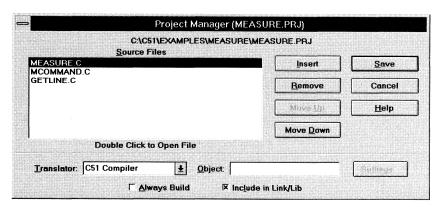
The Project Manager dialog box shows the source files that compose the MEASURE project. There are three source files in this project.
