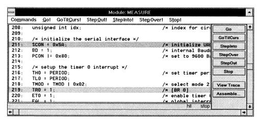
Click on the Go button and dScope starts execution from the current program counter and stops when the breakpoint is reached. To remove a breakpoint, double-click on the line containing the breakpoint.
