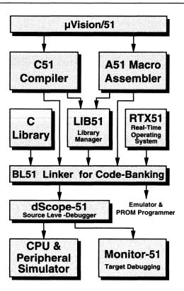
As shown in this figure, files are created by the  $\mu$ Vision/51 IDE and then passed to the C51 compiler or A51 assembler. The compiler and assembler process source files and create relocatable object files.
