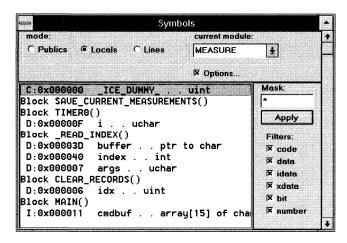
dScope supports the drag and drop feature of Windows and lets you access the symbols this way. Use the mouse to drag and drop the **idx** symbol from the symbol browser window to the command window. The fully qualified symbol name with module name and function name are inserted as shown. The qualifiers are separated by the backslash character ('\'). Select the command window and press **Enter**. dScope displays the value of **idx**.
